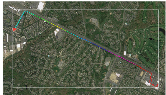
Fig. 4. An illustration of the tight rectangle encapsulating an example route. The rectangle is created by fitting the route in between the minimum and maximum ( latitude, longitude ) pairs of the given route. The minimum and maximum ( latitude, longitude ) pairs correspond to the bottom left (i.e., South West) corner and the top right (i.e., North East) corner of the rectangle, respectively.
