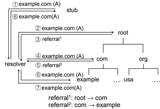
Fig. 1: A workflow of the DNS operation.
