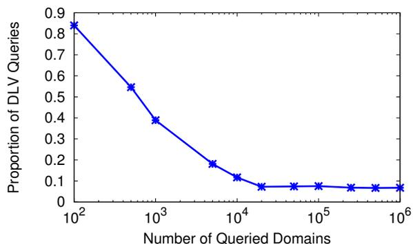
Fig. 9: Proportion of leaked domains. Notice the linear decay (x-axis in log-scale) in the proportion of DLV queries as the number of domains increases, which is understood by the uniformity of the negative caching effect.
