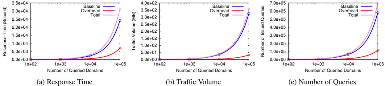
Fig. 10: Baseline, overhead, and total performance in terms of response time (measured in seconds), the total traffic volume (measured in megabytes), and the number of queries. The baseline corresponds to the case when not using the remedies, whereas the overhead is the actual cost of the remedy.
