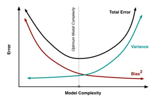
The variation of Bias and Variance with the model complexity. This is similar to the concept of overfitting and underfitting. More complex models overfit while the simplest models underfit.
