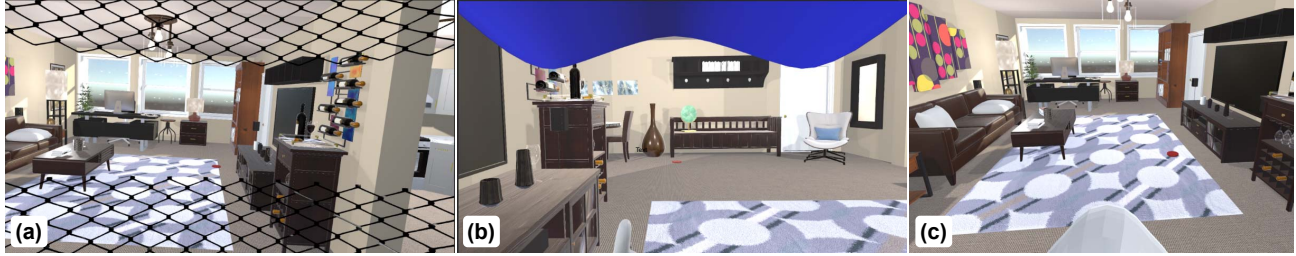
Figure 1: Head-Centric Rest Frames used in the study: (a) - mesh mask, (b) - baseball hat, (c) - virtual nose.
