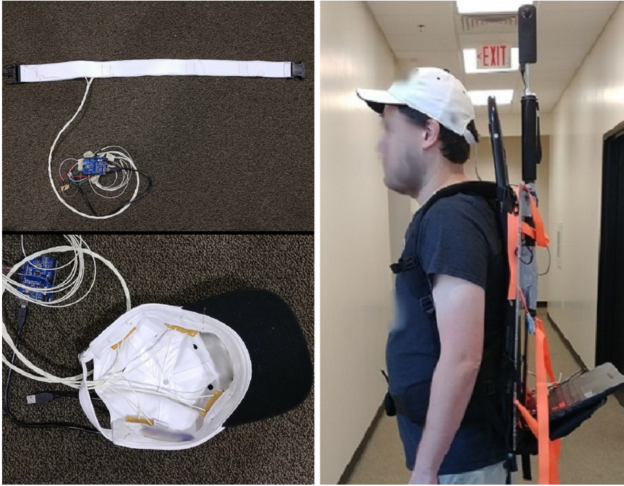
Fig. 1. Left: The developed tactile belt (top) and hat (bottom). Each utilized a 4-tactor design in order to provide feedback to the Streamer. The motors were controlled by an Arduino Uno. Right: A user wearing the backpack rig, which consisted of a 360 camera for livestreaming, a vibro-tactile device for feedback, and a laptop.
