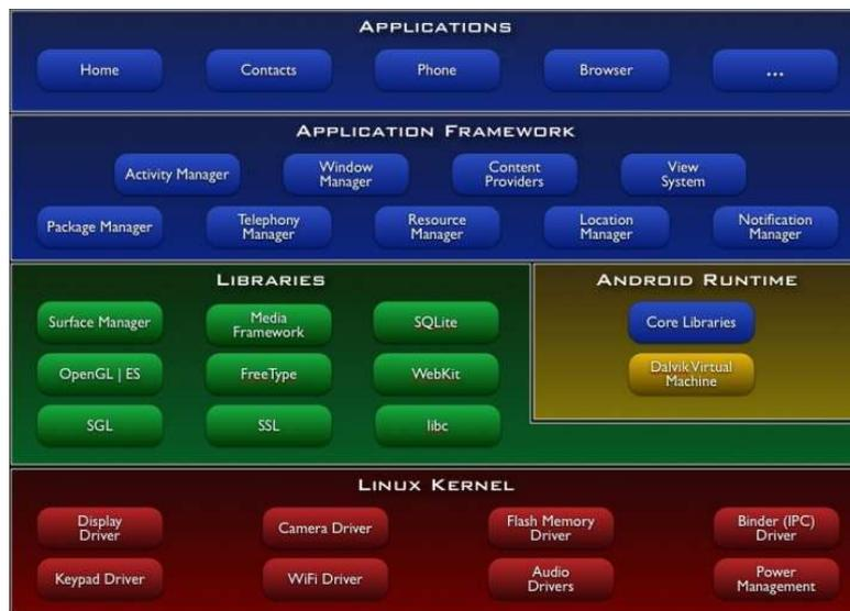
Figure 1: Android System Architecture
