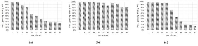
Fig. 6: The ratio between the number of password guessing trails to the total number of all wireless sessions (WS) for (a) Dlink-DIR890L, (b) ASUS-RT-AC68U (c) Linksys WRT54.
