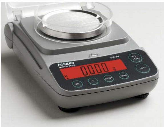
Figure 4.9: Picture of an acculab vicon portable digital balance VIC-303 5
