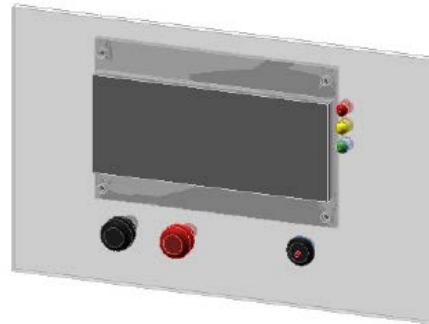
Figure 4.27: SolidWorks model of the user interface panel with components attached
