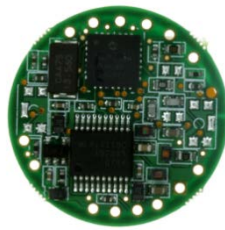
Fig. 5: The small RFID reader is integrated into the bottom-side of the scale-top pane for reading medicine identification and dosage data. It is only 25.4mm in diameter and 2.8mm in height.
