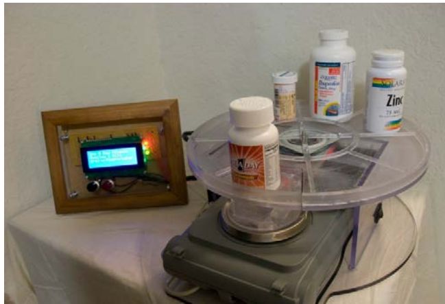
Fig. 3: Picture of our actual RMAIS prototype. The LCD panel on the left displays the medicine name and dosage information of the bottle currently on the scale-top pane. The scale has a dimension of 6.8 x 3.7 x 9.8 inches.
