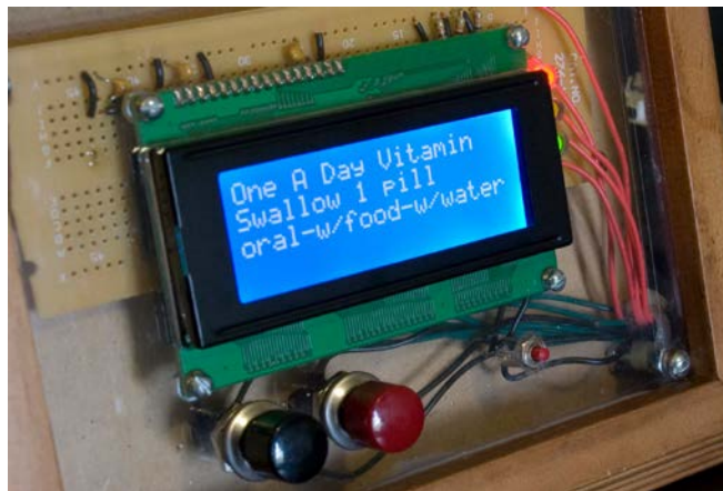
Fig. 6: Picture of the user interface panel ready to administer a medicine. The LCD screen shows the medicine name, dosage, and special instructions for the medication. It can be designed with a large LCD panel to show very large and bright colored text in order to help vision impaired (such as elderly) patients to read.
