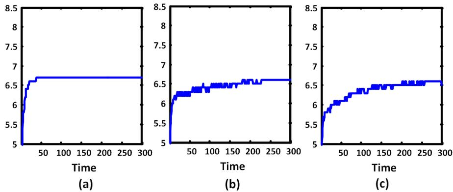
Figure 5: Comparison of CE when  $k \geq n$  and number of networks is kept fixed. Y-axes represent expected utility per CRN. (a)  $k = n = 4$ , (b)  $k = 5, n = 4$ , (c)  $k = 6, n = 4$ . CRNs always select the best out of the available pool of channels therefore the convergence value of expected utilities are equal however convergence rate increase as  $n \rightarrow k$ .
