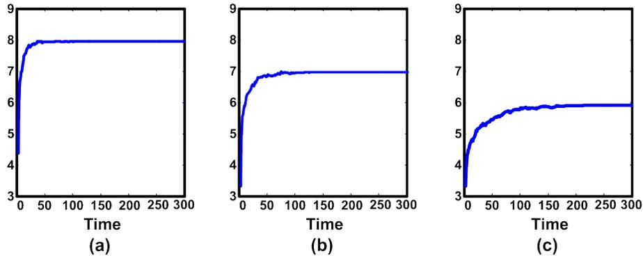
Figure 8: Comparison of CE values when channel payoffs (quality of channels) are varied. Y-axes represent expected utility per CRN with  $k = n = 2$ , (a)  $u_1 = 9, u_2 = 7$ , (b)  $u_1 = 9, u_2 = 5$  and (c)  $u_1 = 9, u_2 = 3$  Decrease in the quality of channel 2 results in a proportional decrease in the expected utility for every CRN. Also, the convergence rate decreases as the variance in channel quality increases.
