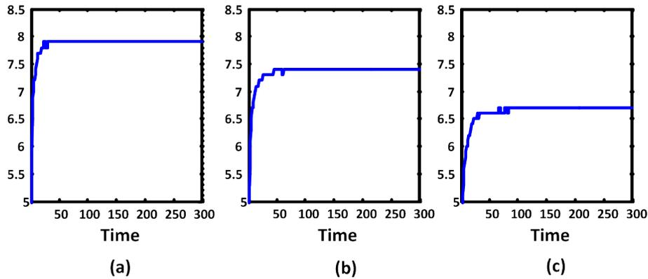
Figure 4: Comparison of CE at different values of the number of networks ( $n$ ) and channels ( $k$ ). Y-axes represent expected utility per CRN. For this simulation  $n = k$  where (a)  $n = k = 2$ , (b)  $n = k = 3$ , (c)  $n = k = 4$  such that  $u_1 = 9$ ,  $u_2 = 7$  and  $u_3 = 6$ .
