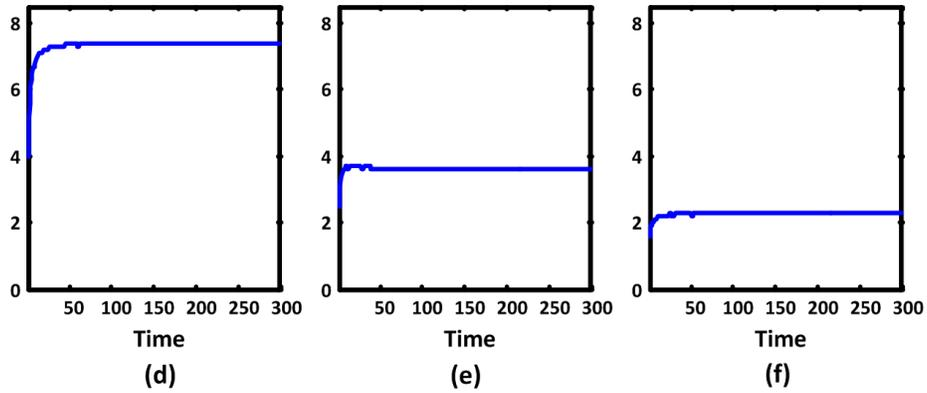
Figure 7: Comparison of CE when  $n \geq k$  and number of channels is kept fixed. Y-axes represent expected utility per CRN. (d)  $k = n = 2$ , (e)  $k = 2, n = 3$ , (f)  $k = 2, n = 4$ . Increase in number of networks results in a corresponding decrease in expected utility per CRN however the convergence rate decreases as the number of channels increases.
