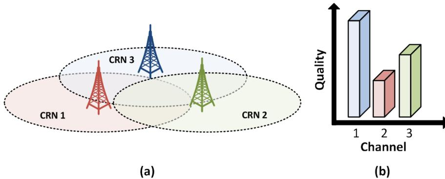
Figure 1: (a) Collocated CRNs competing for (b) Heterogeneous channels. The channels of the spectrum band may vary in quality with respect to availability, bandwidth or SNR, etc.
