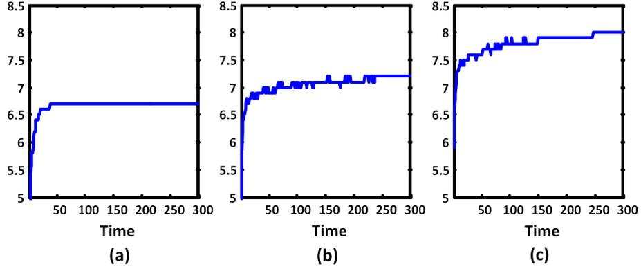
Figure 6:  $n \leq k$  and number of networks is kept fixed. Y-axes represent expected utility per CRN. (a)  $k = n = 4$ , (b)  $k = 3, n = 4$ , (c)  $k = 2, n = 4$ . Decrease in number of networks results in an increase in expected utilities. Convergence rate decreases as the number of channels increases.
