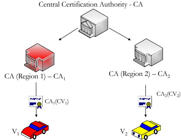
Figure 4.1: A certification authority hierarchy with two regional CAs. CA (Region 1) issues certificates to vehicles registered with in its region, for example certificate CV<sub>1</sub> is issued to vehicle V<sub>1</sub>. (Note: CA<sub>x</sub>(CV<sub>y</sub>) is a certificate issued to vehicle y by a CA of region x.)
