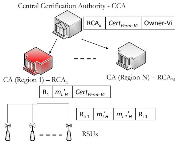
Figure 4.10: Certificate Architecture: CCA maintains current RCA and permanent certificate to owner link, RCA maintains permanent certificate to blinded-long-term certificate link and RSU that reported usage of long-term certificate, each RSU maintains authenticating-certificate (and its issuer) to blinded-short-term certificate link and the RSU that reported usage of issued short-term certificate.
