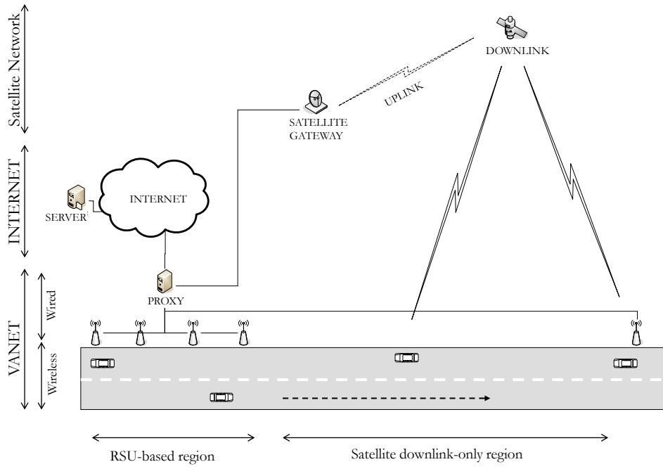
Figure 3.3: Proposed design in context of higher level vehicular network architecture
