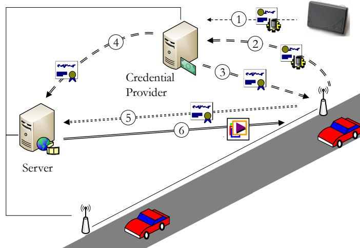
Figure 4.6: Extended services architecture (1) User registers payment device with Credential provider (2) User sends payment/service request (3) Credential provider issues temporary credentials (4) Credential provider informs Server of service purchased and temporary credentials (5) User requests service using temporary credentials (6) Server delivers content.
