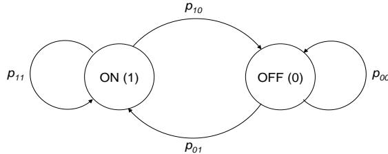
Figure 3.1: Two-state ON/OFF Land Mobile Satellite Channel (LMSC) Model
