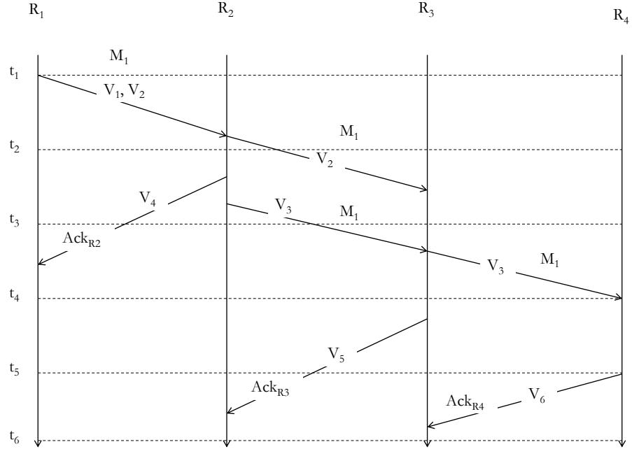
Figure 2.2: Flow of a message and its acknowledgement between  $\text{RSU}_1$  and  $\text{RSU}_4$  (illustrated also in Figure 2.3). Message  $M_1$  is sent from  $\text{RSU}_1$  to  $\text{RSU}_4$  via  $\text{RSU}_2$  and  $\text{RSU}_3$ .  $t_i$  represents time in order.  $R_i$  represents  $\text{RSU}_i$ .  $V_i$  represents vehicle  $i$  that carries a message.  $\text{Ack}_{R_i}$  is the acknowledgement message from  $\text{RSU}_i$  to  $\text{RSU}_{i-1}$ .
