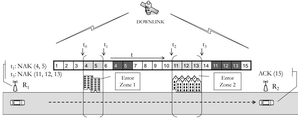
Figure 3.7: Error location prediction and avoidance. The system predicts the segments which may have been lost on the bases of previous data and proactively retransmits these segments.
