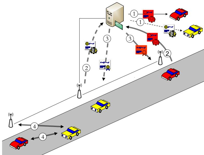
Figure 4.4: Architecture (1) Users register their payment devices with Provider beforehand (2) Users send payment/service requests (3) Provider issues temporary credentials (4) Users participate in VANET via vehicle to vehicle or vehicle to infrastructure communication.
