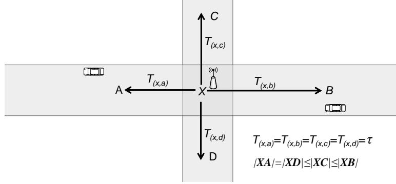
Figure 5.11: Balloon expansion: The expansion is independent along each direction and depends on vehicle speed, vehicle density, event/incident distribution and probability of vehicles following a route.  $|XA|$ ,  $|XD|$ ,  $|XC|$ , and  $|XB|$  gives the size of expansion towards A, B, C and D respectively for  $\tau$  average reporting time over each route.
