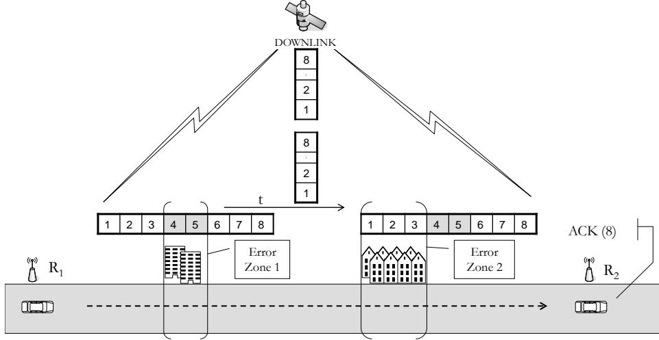
Figure 3.6: Repeated transmission, whole data set is repeated several times. Data segment(s) lost can be recovered from later repeated transmissions.
