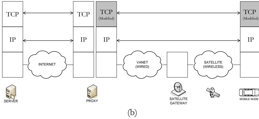
Figure 3.4: Protocol stacks for different regions. (a) Content transfer to mobile node via Road side units. (b) Content transfer to mobile node via satellite.
