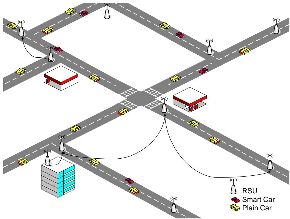
Figure 2.1: The proposed architecture consists of RSUs deployed along the roads. RSUs can be standalone (the three RSUs on top right), locally connected to adjacent RSU (two on the up-left corner), or connected to Internet infrastructure (three on the bottom). What versions of RSUs to install depends on overall budget and services we want to provide.
