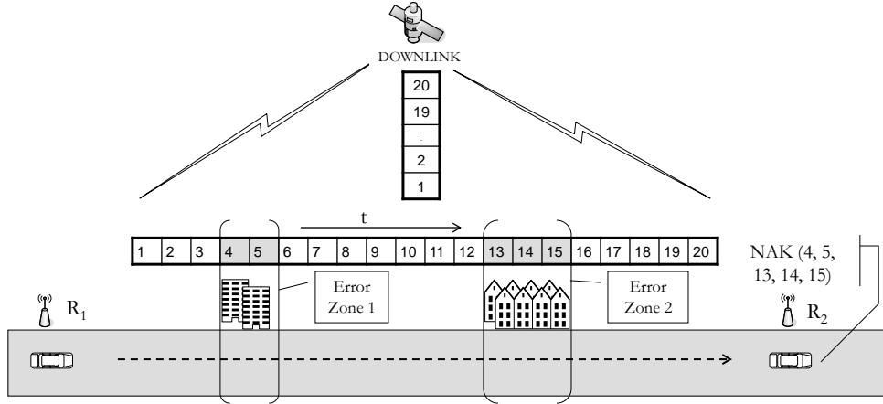
Figure 3.5: Baseline architecture, delivery of content takes place through satellite while the mobile node is traveling between R<sub>1</sub> and R<sub>2</sub>. The mobile node sends NAK for the lost segments when reaching R<sub>2</sub>, where R<sub>2</sub> takes charge and resends these lost segments to the mobile node.
