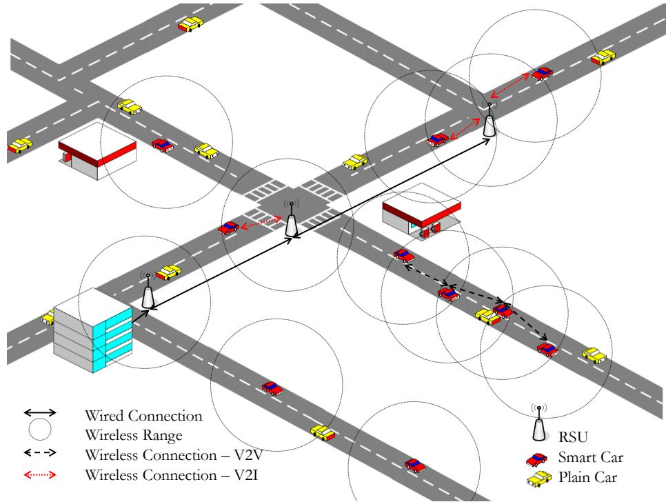
Figure 1.1: Vehicular ad hoc network - VANET
