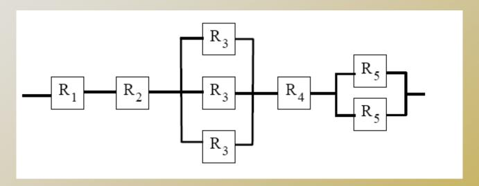
$$R_{sys} = R_1 \cdot R_2 \cdot [1 - (1 - R_3)^3] \cdot R_4 \cdot [1 - (1 - R_5)^2]$$
