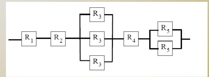
$R_{sys} = R_1 \cdot R_2 \cdot [1 - (1 - R_3)^3] \cdot R_4 \cdot [1 - (1 - R_5)^2]$
