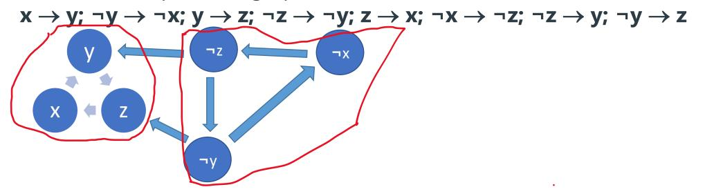
b. Draw circles around the strongly connected components (see red circles) c. Provide a solution based on the SCCs or highlight the conflict exposed by the SCCs – the cluster with three elements has no outgoing edges, so  $\mathbf{x} = \mathbf{y} = \mathbf{z} = \mathbf{T}$
