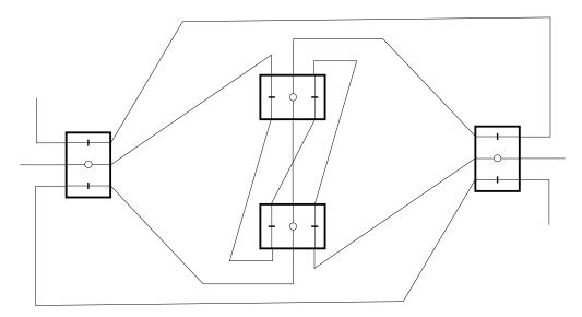
Figure 11: A crossover constructed from stacked tripwire-lock-tripwires
