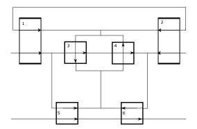
Figure 6: 2-toggles simulate 1-toggle-lock.
