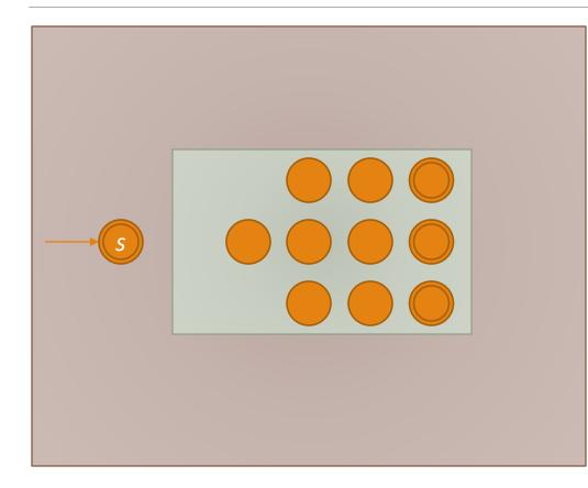
Let  $N_A = \{ Q_A, \Sigma, \delta_A, q_{0A}, F_A \}$  be an NFA recognizing regular language A. Construct a new NFA  $N = \{ Q, \Sigma, \delta, s, F \}$  with:  $\circ Q = Q_A \cup \{ s \}$  $\circ$  Start state s  $\circ F = F_A \cup \{ s \}$
