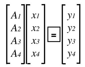
Compute each vector element in parallel by partitioning.
