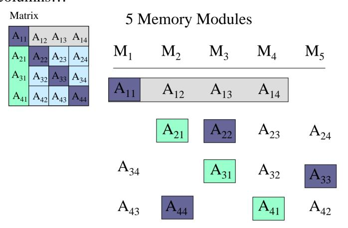
At the cost of adding another memory module and wasted space, we can now access the matrix in parallel by row, column, and main diagonal.
