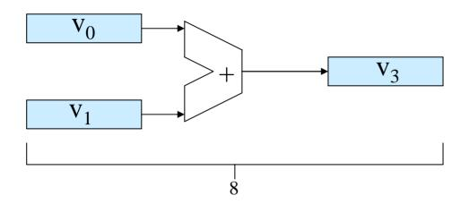
Using pipelining it takes 8 units of time to fill pipeline and produce first result, each unit of time after that produces another result  $T_{p+} = 8 + 63$
