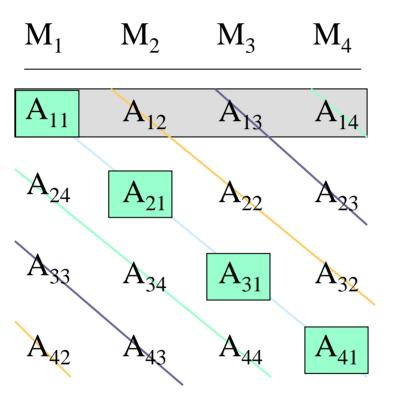
By using a skewed matrix representation, we can now access each row and each column in parallel.
