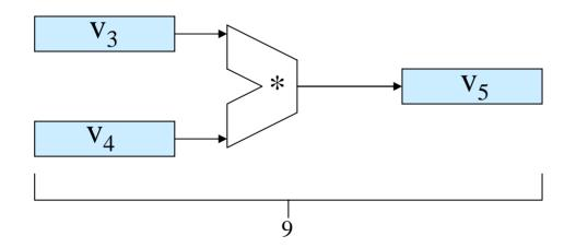
The multiplication pipeline takes 9 units of time to fill, and produces another result after each additional unit of time
