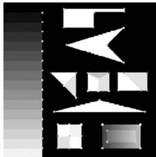
Output of the SUSAN corner detector ( t=10 ) given the test image. (0.3 sec)
