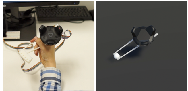
(b) Physical grabber controller (Left) and virtual grabbers (right) when closing the chopsticks on a virtual object. Note that the physical grabbers close in conjunction with the virtual grabbers grabbing onto the virtual object to provide the expected force feedback.
