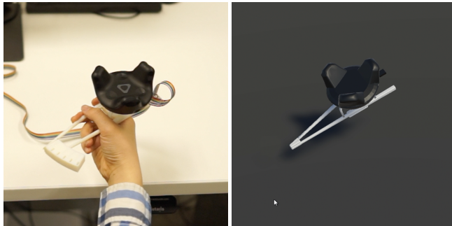
(a) Physical grabber controller (Left) and virtual grabbers (right) when closing the grabbers with no virtual object in between. Note that the physical grabbers close in conjunction with the virtual chopsticks as expected.
