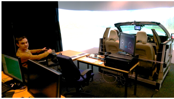
Figure 5. The driving simulator and the WOZ driver acting as the vehicle automation in Case Study A . The WOZ assistant providing interface feedback was seated to the right of the wizard driver (empty chair).
