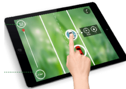
Figure 7. Illustration of the final controller design in Case Study C that enables drivers to issue tactical commands to highly automated vehicles.
