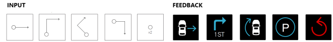
Figure 3. Finger gestures (left) and visual feedback in the instrument cluster (right) in Controller II .
