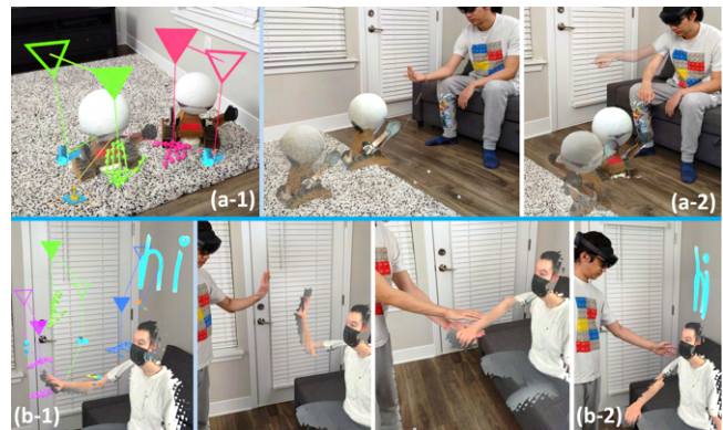
Figure 12: (a) An interactive toy robot: (a-1) A planar joint is connected to the robot. A 'come' dynamic gesture is connected to a 'moving' animation action as a dynamic-provoking interaction , while a 'pointing' dynamic gesture is demonstrated referring to a 'rotation' animation as a synchronous interaction . (a-2) The toy robot can move towards the user after the user does a 'come' gesture and rotates synchronously with the user's 'pointing' hand command. (b) A humanoid agent: (b-1) Two spherical joints link the agent's body, upper, and lower arm. A double-handed static gesture is created next to the agent's hand and connected with a following action . A 'waving hand' dynamic gesture is connected with a similar 'waving hand' animation action of the agent. A sketched "Hi" is linked with a 'patting' static gesture. (b-2) The virtual agent can wave the hand, shake hands with the user, and pop up a "Hi" after the user pat on the agent's shoulder.
