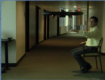
A user controlling an unmanned aerial vehicle (UAV) with 3D gestures. (Image courtesy of Joseph LaViola).
