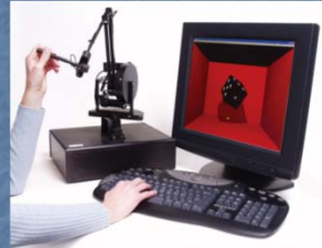
A ground-referenced force-feedback device. (Photograph courtesy of SensAble Technologies)
