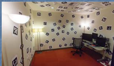
Marker-based inside-out tracking system that uses several fiducial markers with known unique patterns placed strategically on the walls and ceiling of a room. (Photograph courtesy of Valve)
