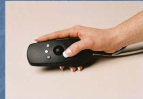
The Wanda input device containing a 6 DOF tracker, three buttons and an isomorphic ball. (Photograph courtesy of Ascension Technology Corporation)
