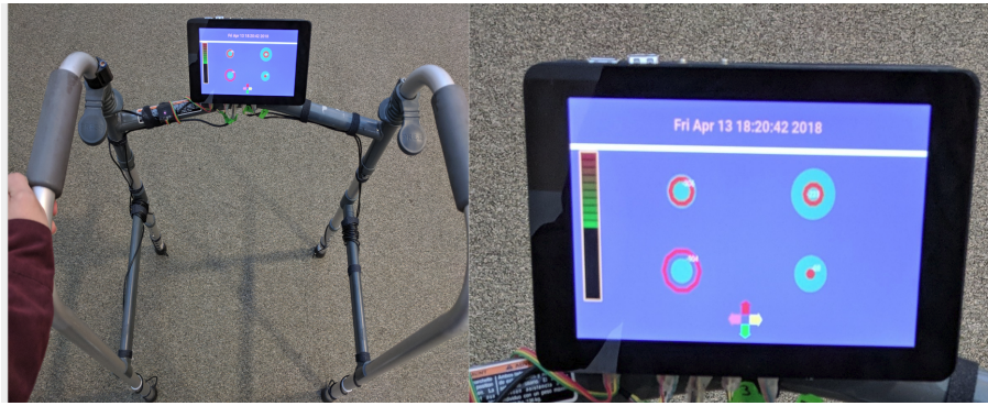
Figure 1: The IoT augmented walker from the point of view of the user (left) and a close-up of the screen (right). The user is applying more weight to the left side of the walker.
