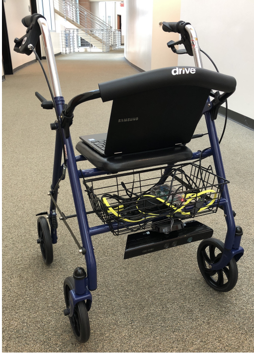
Fig. 1. The smart walker configured for the point cloud processing approach.
