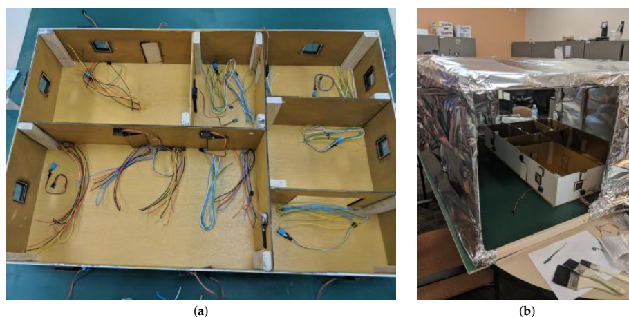
Figure 1. (a) The layout of the ScaledHome-2 testbed. (b) The testbed in the environmental enclosure.
