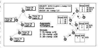
Figure 2: A sensor network (left) with an in network, grouped aggregate applied to it (right). Parenthesized numbers represent nodes that contribute to the average
