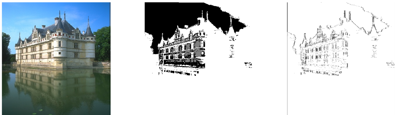
Figure 3: Results of Kmeans clustering with normalized feature vectors, features obtained by using Gaussian filters of different scales : Original image (on the left), Kmeans cluster assignment on image pixels (in the middle) and boundary extracted from the k-means cluster (to the right)
