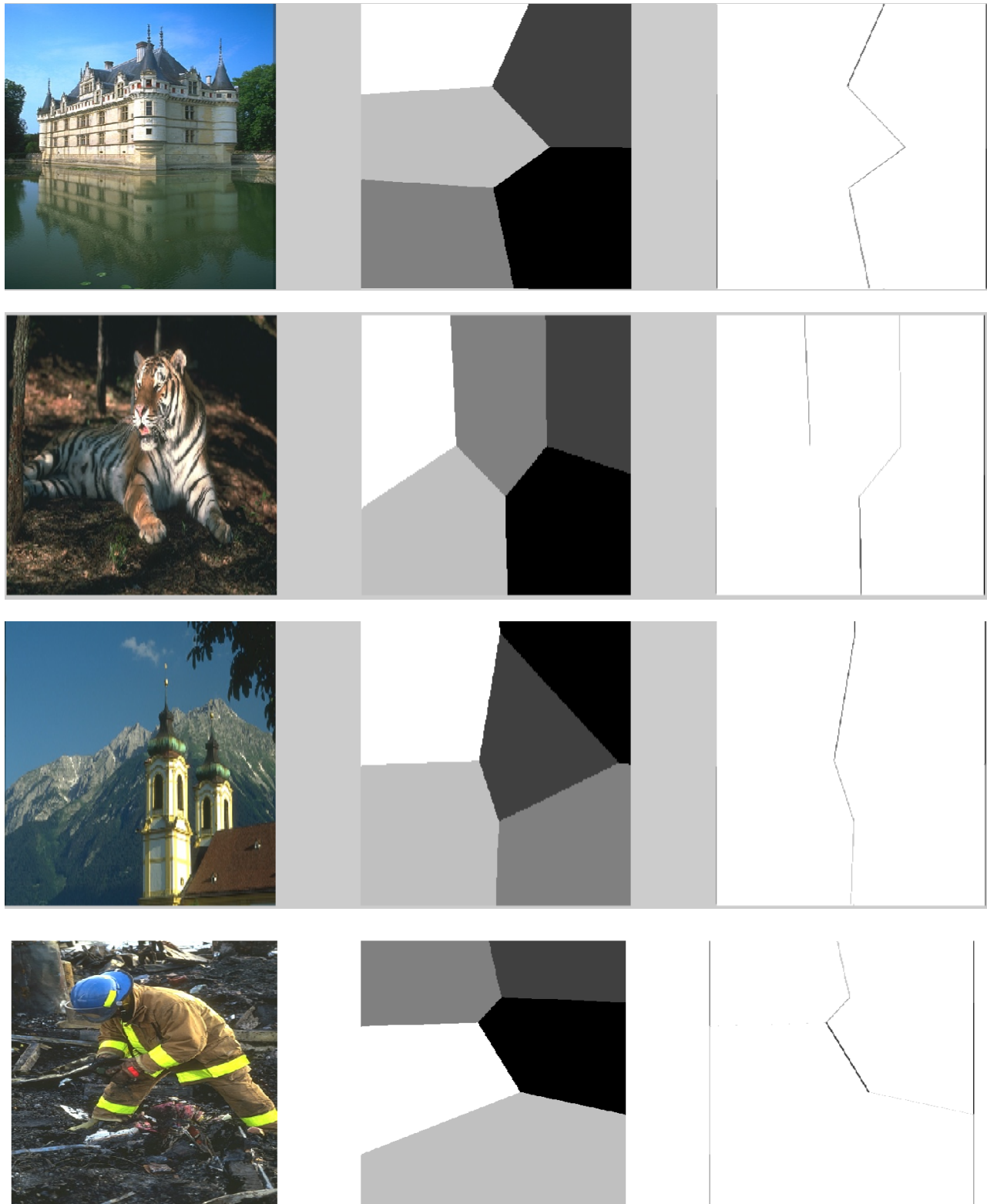
Figure 1: The above figures depict how the kmeans clustering algorithm performs on the original image (on the left), Kmeans cluster in the middle and boundary extracted from the k-means cluster (to the right)
