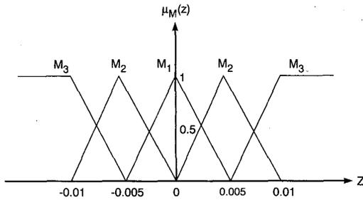
Fig. 1 Symmetric triangle membership function
