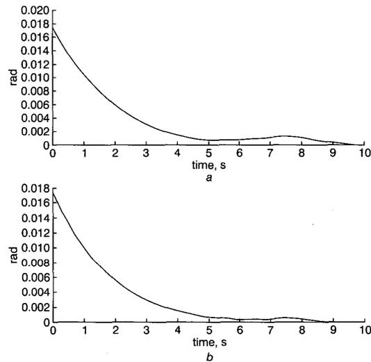
Fig. 3 Position errors (a)  $e_1$  and (b)  $e_2$  under robust fuzzy control
