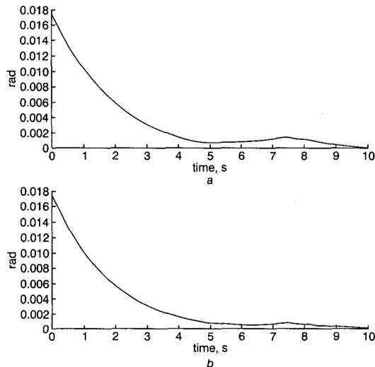
Fig. 2 Position errors (a)  $e_1$  and (b)  $e_2$  under robust control
