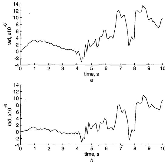
Fig. 4 Comparison of tracking performance,  $e_{\text{robust}} - e_{\text{fuzzy}}$
