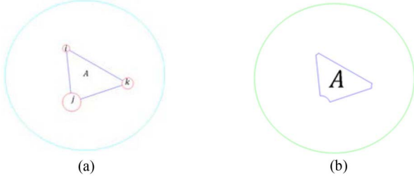
Fig. 9. RT A , with and without disks, to be observed from a CP P(A) . (a) RT forms by disks i, j , and k . (b) Diskless region A is visible from every point on P(A) .
