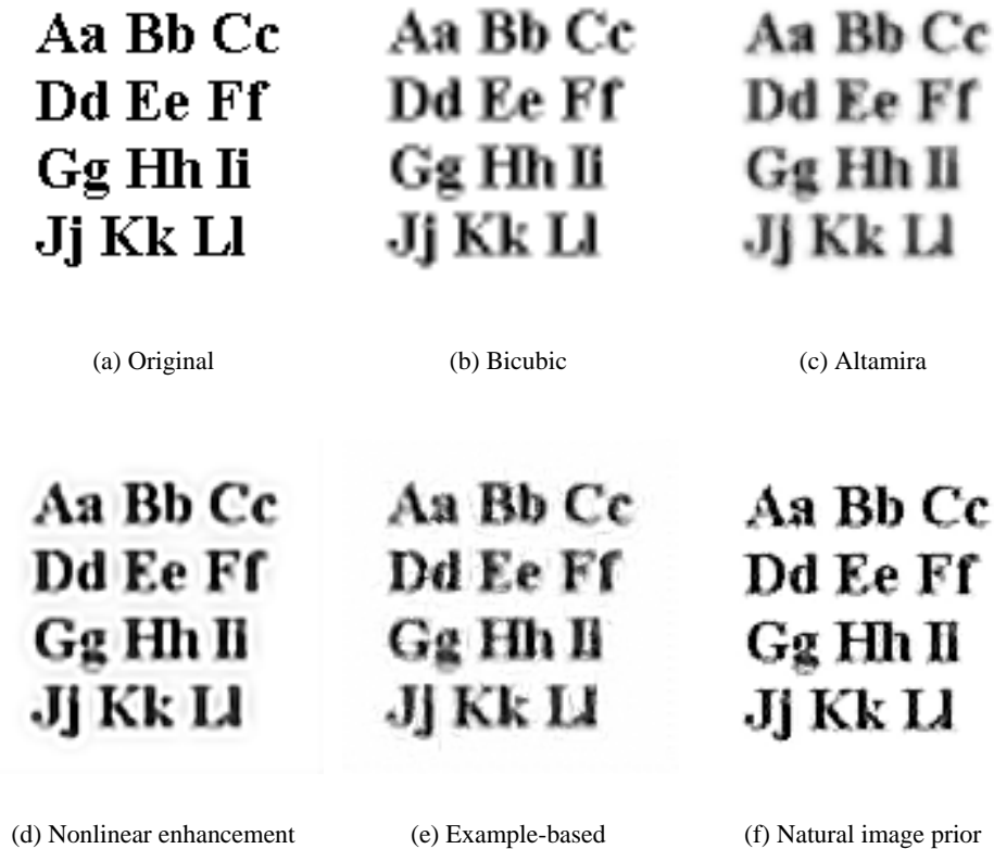
Figure 9: 128 \times 128 synthetic font image (not included in the test gallery), decimated to 64 \times 64 and then super resolved [MSE in brackets]. (a) True high resolution; (b) Bicubic interpolation [0.0345]; (c) Altamira [0.0294]; (d) Greenspan et al. nonlinear enhancement [0.0740]; (e) Freeman et al. example-based [0.0599]; (f) our natural image prior based algorithm [0.0133]. As in Figures 7 and 8, we see that our algorithm produces a sharp result. Moreover, notice that the nonlinear enhancement algorithm has significant “haloing” artifacts around the fonts. These artifacts do not appear in our outputs.
