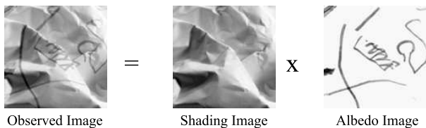
Figure 1. An example of how an image of crumpled paper with scribbling on it can be expressed as the product of two intrinsic component images, a shading image and an albedo image.
