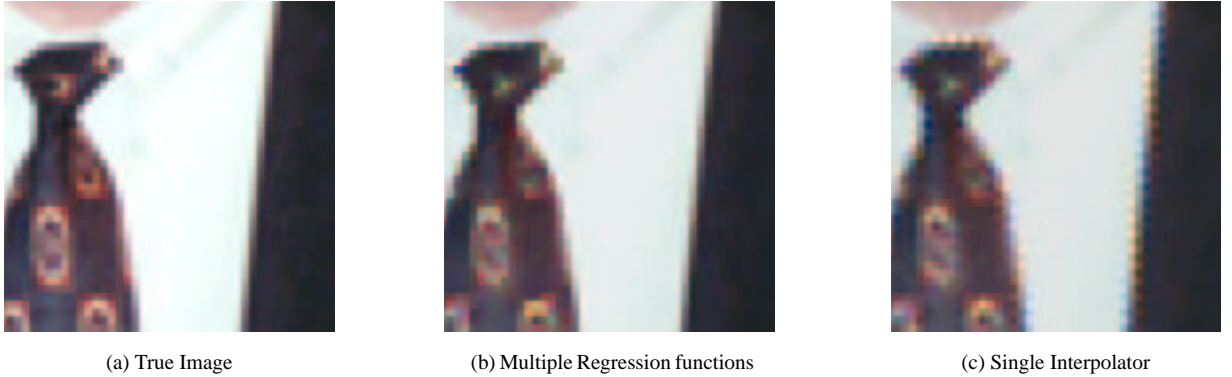
Figure 6: A comparison of the results produced by using multiple interpolators versus a single interpolator. Notice that the image produced with multiple interpolators, shown in (c), does not have the color fringes along the coat and tie.
