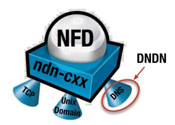
Figure 2: DNDN is implemented as a transport face (DNS) within the current NDN architecture.
