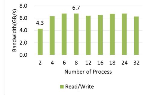
Fig. 7: Read/Write bandwidth in a SMB server
