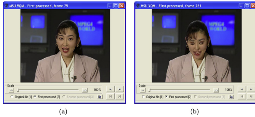
Fig. 10. Processed frames at destination during playback. ANCON could successfully predict playback quality at: (a) Frame-75, when MOS projection was 4.257 (higher quality), and (b) Frame-261 with slight distortions, when MOS projection was 3.25 (mediocre quality).
