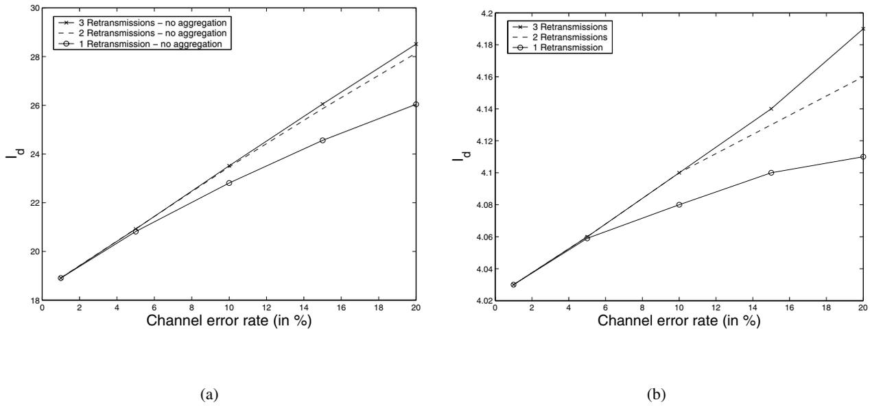
Fig. 9. a) Delay impairment without aggregation; b) Delay impairment with aggregation
