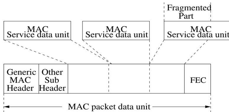
Fig. 2. An MPDU accommodating multiple MSDUs
