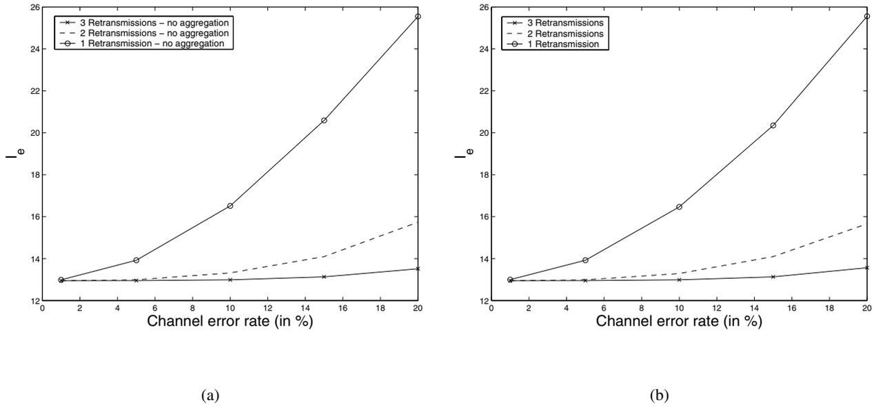
Fig. 8. a) Loss impairment without aggregation; b) Loss impairment with aggregation
