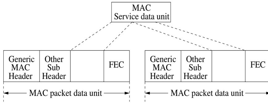
Fig. 3. Single MSDU fragmented to multiple MPDUs
