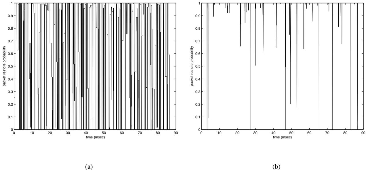
Fig. 5. a) Packet restore probability for non-adaptive scheme; b) Packet restore probability for adaptive scheme
