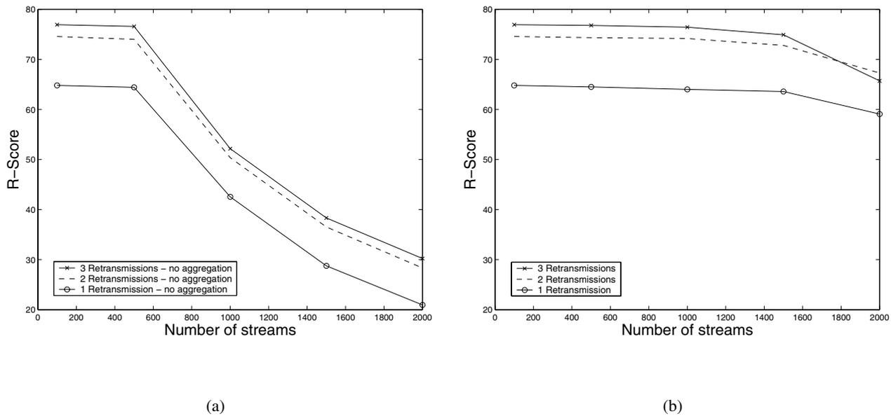
Fig. 11. a) R-score vs. number of streams without aggregation; b) R-score vs. number of streams with aggregation
