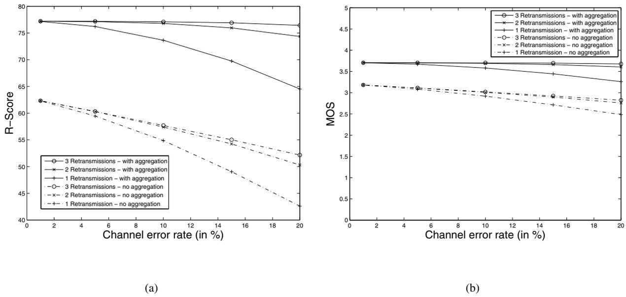
Fig. 10. a) R-score vs. error rate with and without aggregation; b) MOS vs. error rate with and without aggregation
