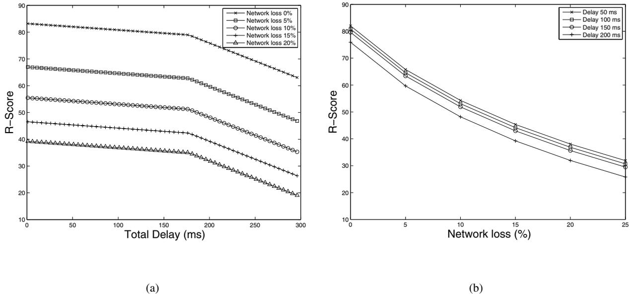
Fig. 4. a) R-score vs. delay; b) R-score vs. network loss
