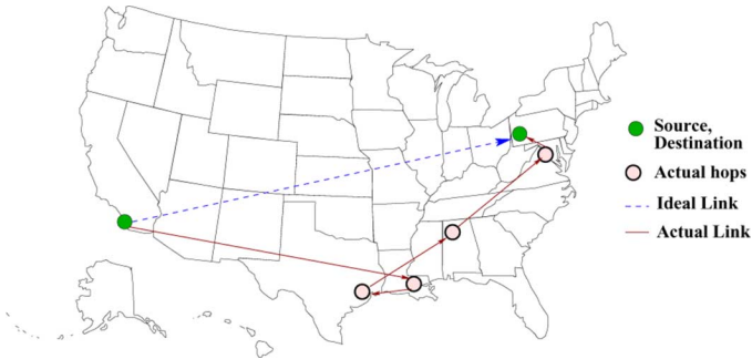
Fig. 9. Ideal path versus actual Internet path for the probe train experiment.
