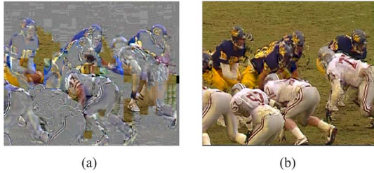
Fig. 8. QoE versus QoS. Both clips experience the same loss rate (QoS), but the QoE is very different: (a) key frame corrupt (low QoE); (b) non-key frame corrupt (higher QoE).
