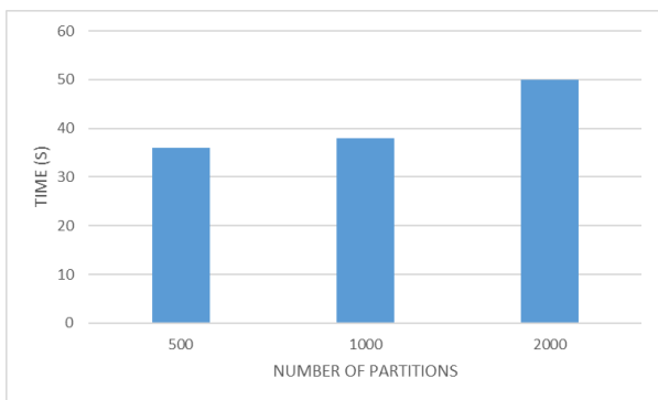
Fig. 11. Performance of different number of partitions with the same data size.
