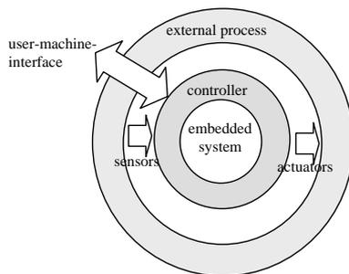
Figure 1. Main components of an embedded system
