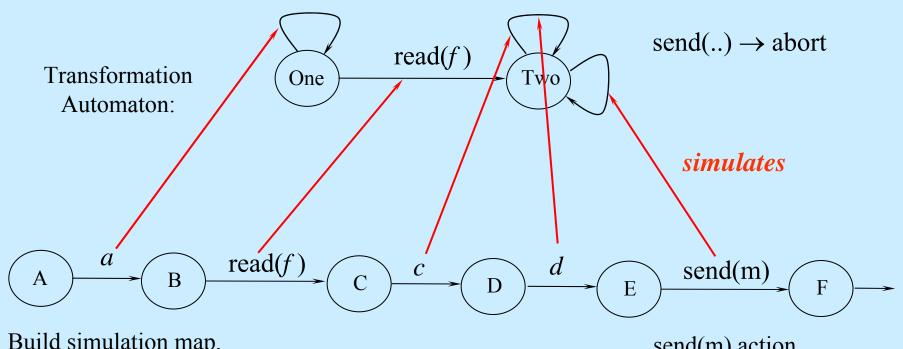
Build simulation map, then generate new code for corresponding actions
