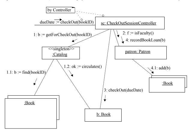
The following is a collaboration diagram for the startCheckOut system operation; it will be used in the next problem. Note that ICheckOutPolicy is an interface.
