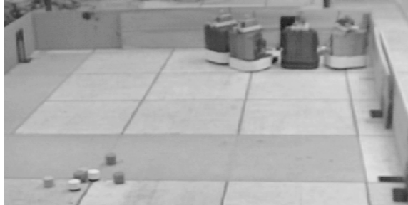
Figure 3: An example of the resting/recharging behavior, triggered by their internal clocks. In this case, the robots have all learned to go home to rest. The figure shows a late stage in the learning, as demonstrated by the small number of remaining pucks.
