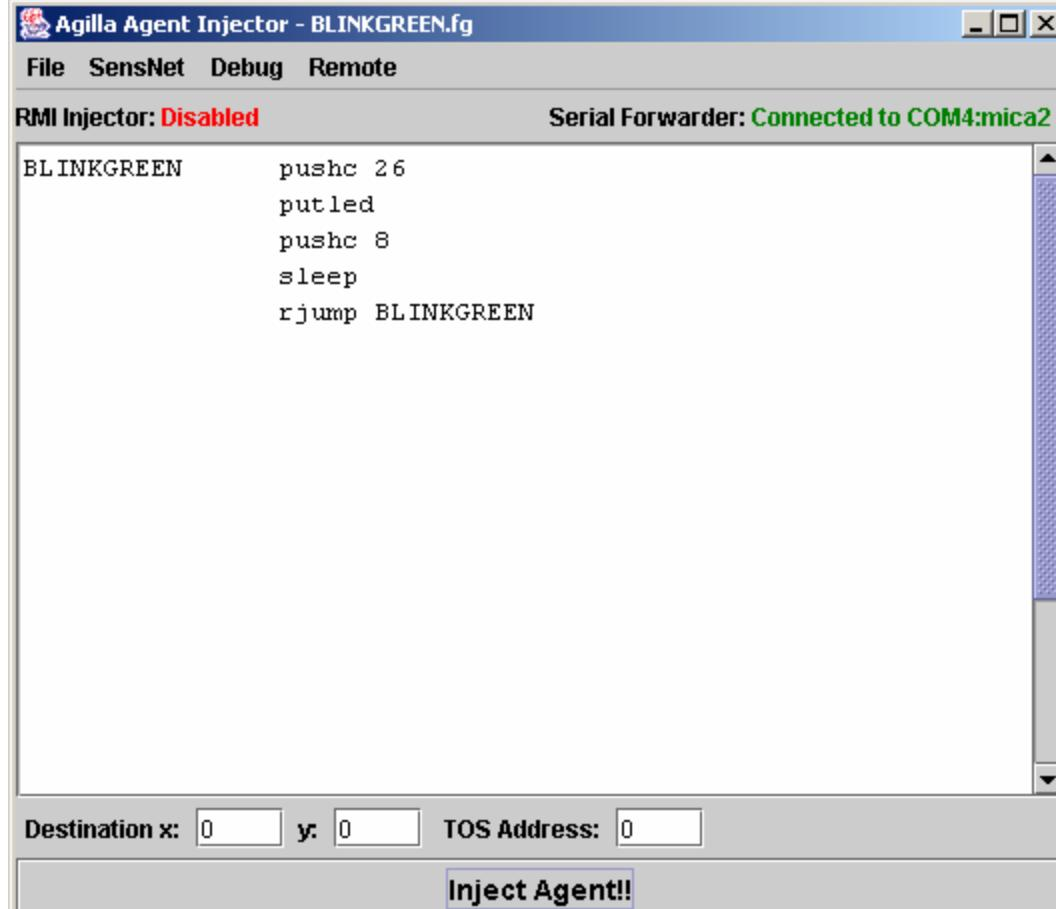
The screenshot shows the Agilla Agent Injector interface with the title bar "Agilla Agent Injector - BLINKGREEN.fg". The menu bar includes File, SensNet, Debug, and Remote. Status indicators show "RMI Injector: Disabled" and "Serial Forwarder: Connected to COM4:mica2". The main window displays assembly code:
