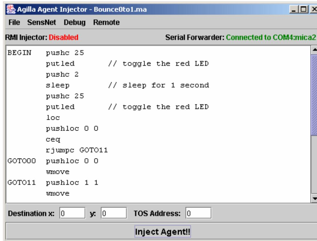
The screenshot shows the Agilla Agent Injector interface with the title bar "Agilla Agent Injector - Bounce0to1.ma". The menu bar includes "File", "SensNet", "Debug", and "Remote". The status bar indicates "RMI Injector: Disabled" and "Serial Forwarder: Connected to COM4:mica2". The main window displays assembly code:
