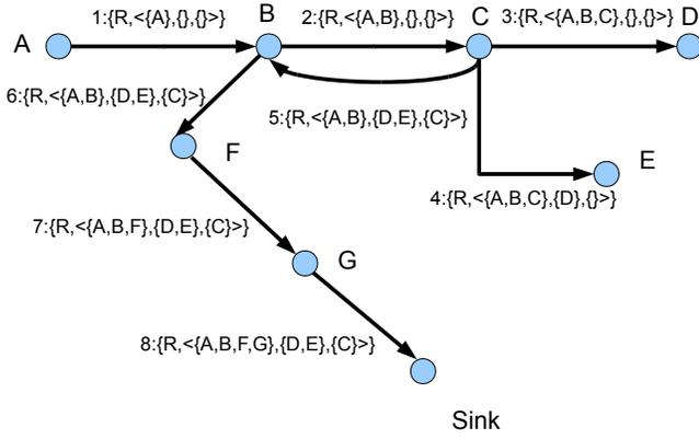
Fig. 1. An example of the path of the report in the TAB protocol.
