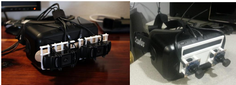
Figure 3. Oculus Rift with original webcams and mounting on the left. Finalized prototype with webcams and improved mounting on the right.
