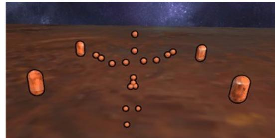
**Figure 1: Example of Fusion System in the Unity scene. Each capsule represents a Kinect camera in the lab and the spheres represent skeleton joints.**
