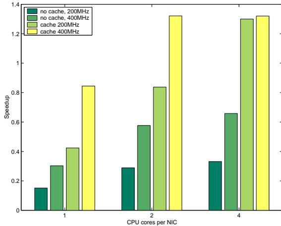
**Figure 4. Speedup of Partitioned Query with Filter and Aggregate**
