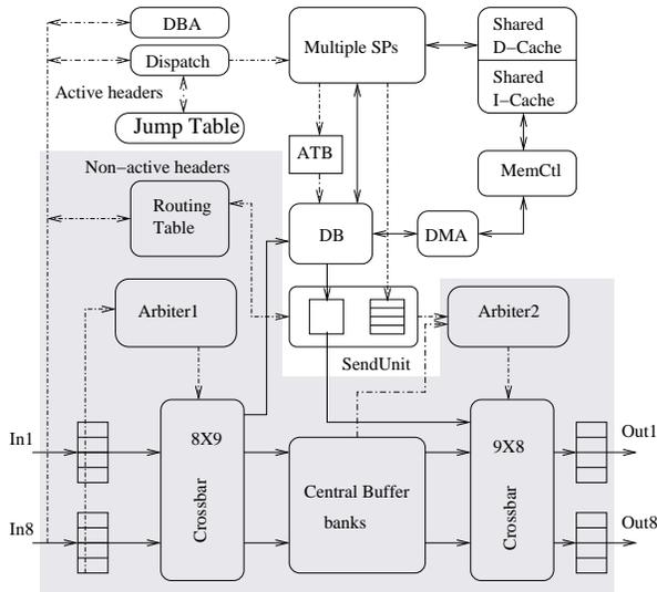
Figure 3. Switch architecture with multiple SPs
