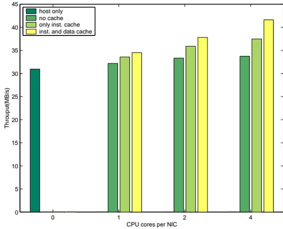
Figure 10. Throughput of Resample Operator
