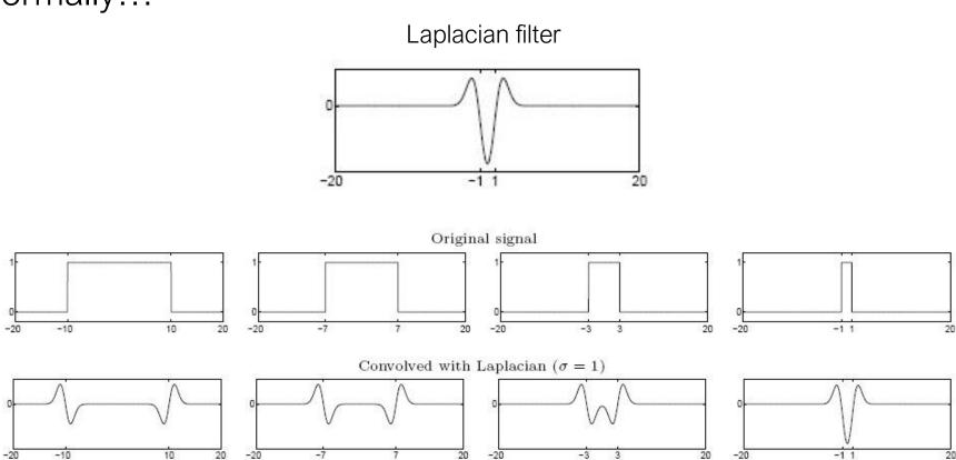
Highest response when the signal has the same **characteristic scale** as the filter
